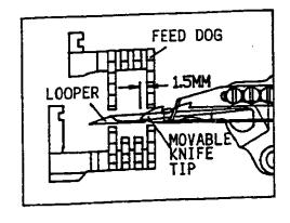
WHEN MOVABLE KNIFE KEEP MOVING TO THE LEFT TILL 1.5mm AWAY FROM THE RIGHT SIDE OF FEED DOG'S LEFT COLUMN, THE TIP OF THE MOVABLE KNIFE SHOULD STILL STAY WITHIN THE RIDGE OF THE LOOPER.
